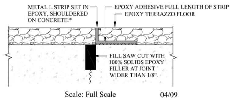
\*Care should be taken by concrete contractor to provide a straight joint, placed in coordination with design teams consideration of final grid pattern. Square edges are encouraged. Tooled edges are discouraged.
